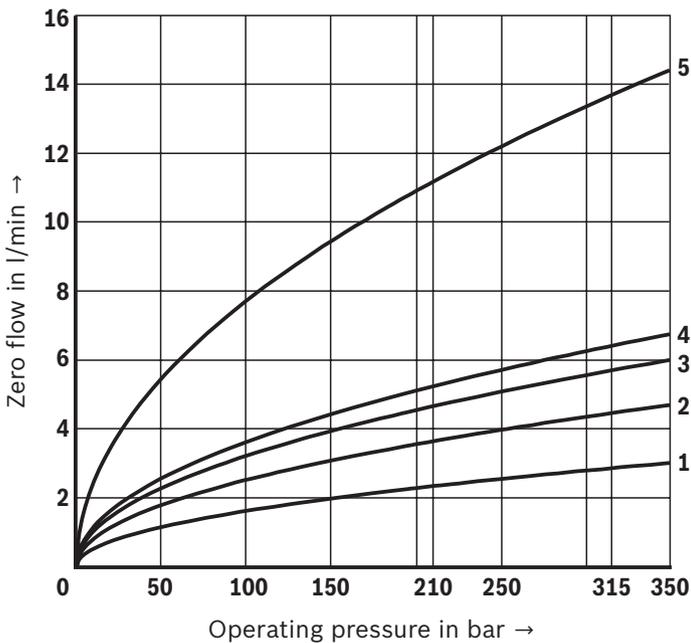
**Maximum internal leakage of the main stage (symbol W) with pilot control valve**
