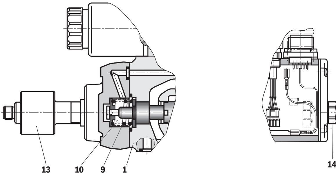
**Pilot oil supply** (schematic illustration)
