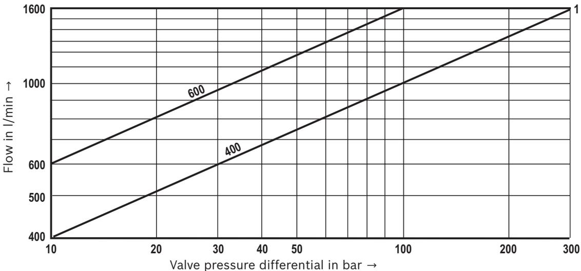
**1** Recommended flow limitation (flow velocity 30 m/s)
