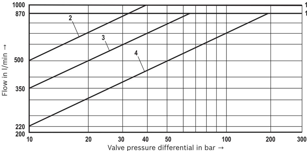
**1** Recommended flow limitation (flow velocity 30 m/s)
