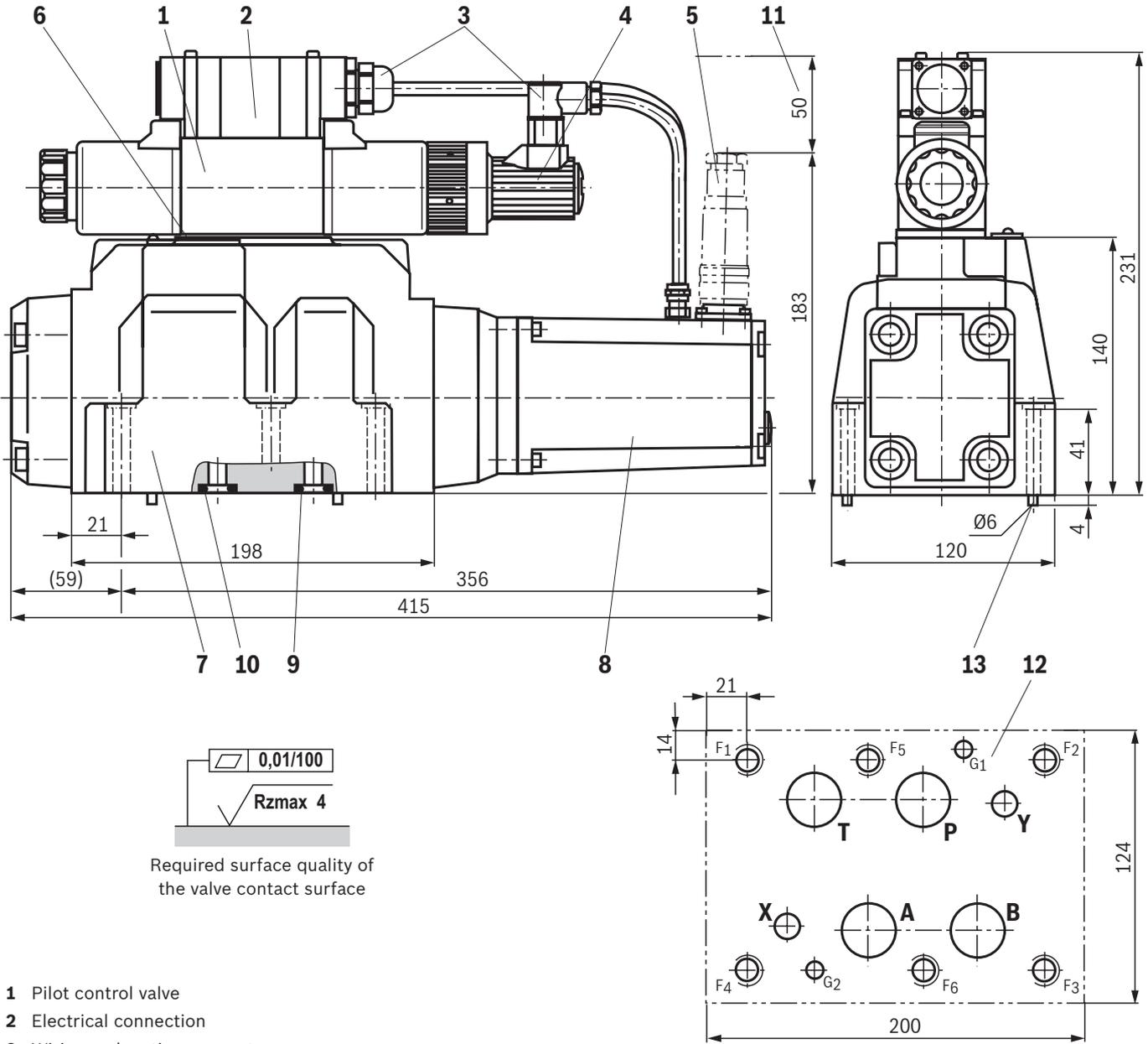
Required surface quality of the valve contact surface
