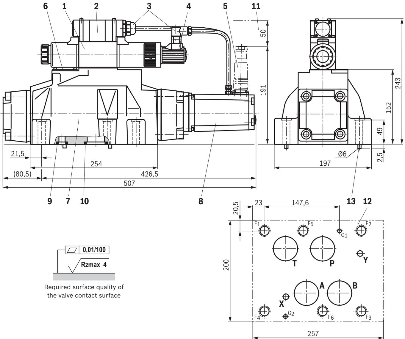
Required surface quality of the valve contact surface
